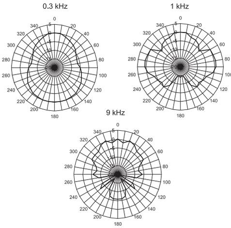
FIGURE 3 Directivity measurements at three frequencies for the loudspeaker used in Experiments 1 and 2.
