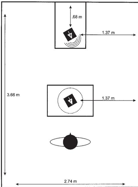
FIGURE 4 Experimental setup used in Experiments 1 and 2. Listeners used the response loudspeaker *r* to indicate the perceived facing angle of the stimulus loudspeaker *s*. The response table was moved between blocks of trials so that the distance between the two loudspeakers was 0.91 m and 1.82 m.
