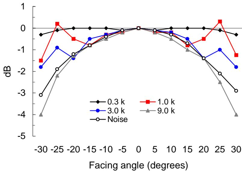
Fig. 1. Loudspeaker directivity measurements 1.5 m from the source at four frequencies and using the broadband noise stimulus.
