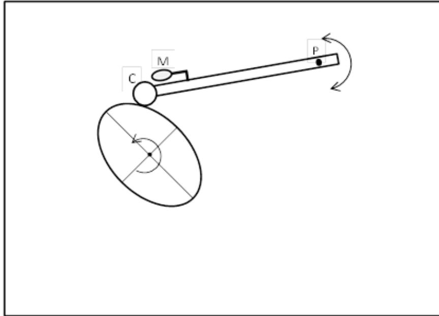
*Figure 1.* Schematic diagram of the recording apparatus. An ellipse attached to the shaft of a motor rotated against a contactor (C), attached to an arm, which pivoted via a ball bearing connection (P), with the contactor in constant contact with the rotating ellipse. A microphone (M), attached to the pivoting arm, picked up the sound made as the ellipse rubbed against the contactor.
